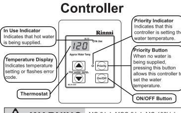
WARNING MC-91-1, MCC-91-1, MC-100V-1, and BC-100V-1 controllers are not compatible with Alternate Temperature Settings. Alternate Temperature Settings are for commercial applications only. DO NOT use the MC-91-1, MCC-91-1, MC-100V-1, or BC-100V-1 controllers when dip switches 2 and 3 (bank of 6) are in the ON position.
